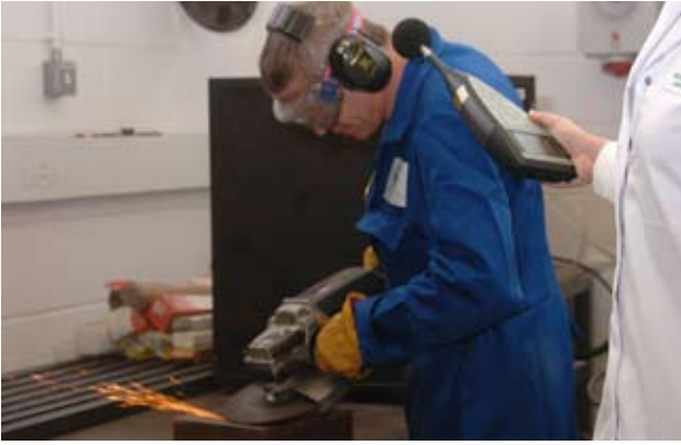
Figure 2.11 Measurement of the sound level by the ear of an operator (Photo © and by courtesy of Health and Safety Executive – Great Britain)
