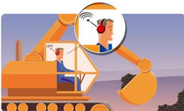
Figure 5.11 At a workstation, where communication is required, a worker uses ear-muffs fitted with electronic communication systems
