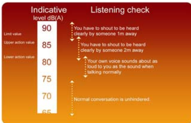
Figure 2.2 Listening checks, indicative steady noise levels and typical sounds
