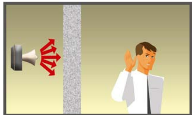
Figure 4.12 Separate noisy equipment by walls
