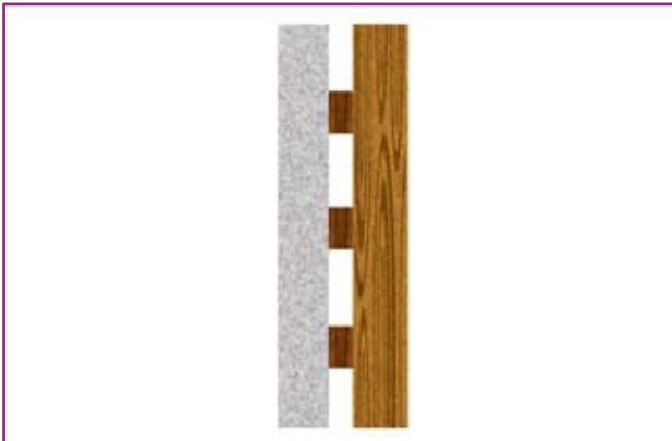
Figure 3.7 'Diaphragms' are wood panels fixed to walls over battens. They attenuate low-frequency sounds
