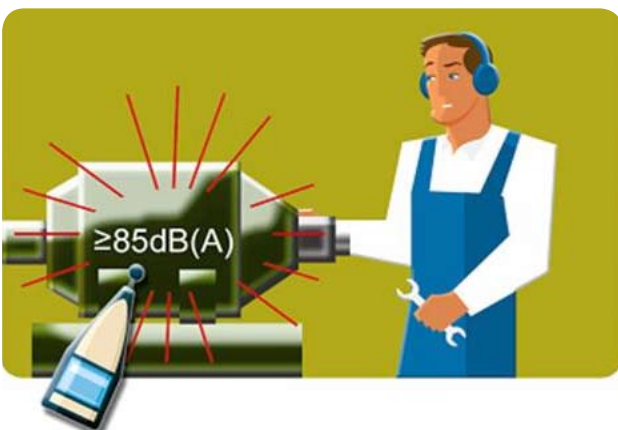
Figure 5.2 Noise exposure matches or exceeds upper exposure action values; workers must use hearing protectors
