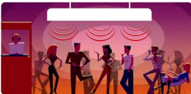
Figure 8.1 Discotheque with acoustic ceiling incorporating several loudspeakers instead of two main loudspeakers
