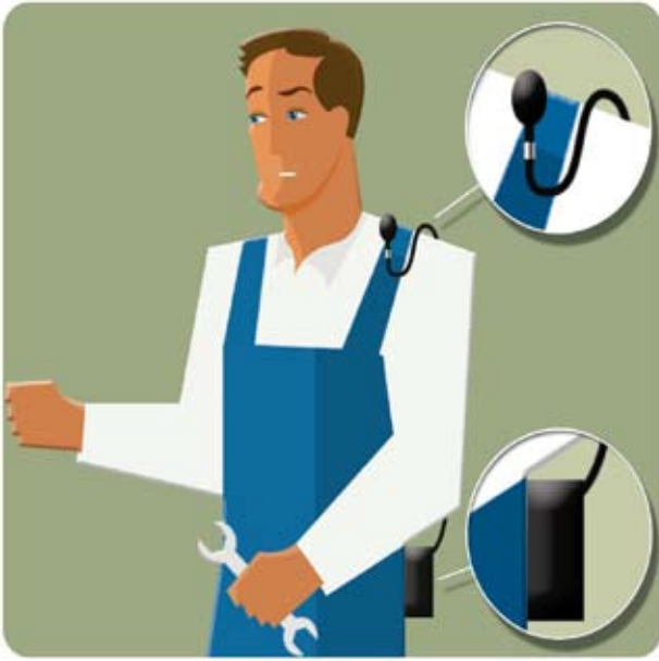
Figure 2.12 Dosimeter microphone positioned on the shoulder
