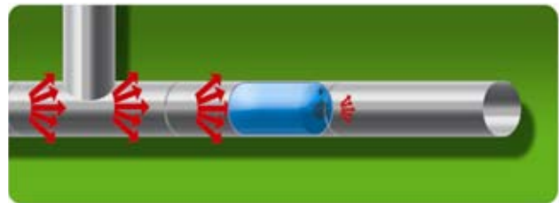
Figure 4.6 Fluid-borne sources: act on flow or use silencers
